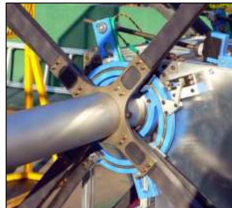
Control device and rotor hub
